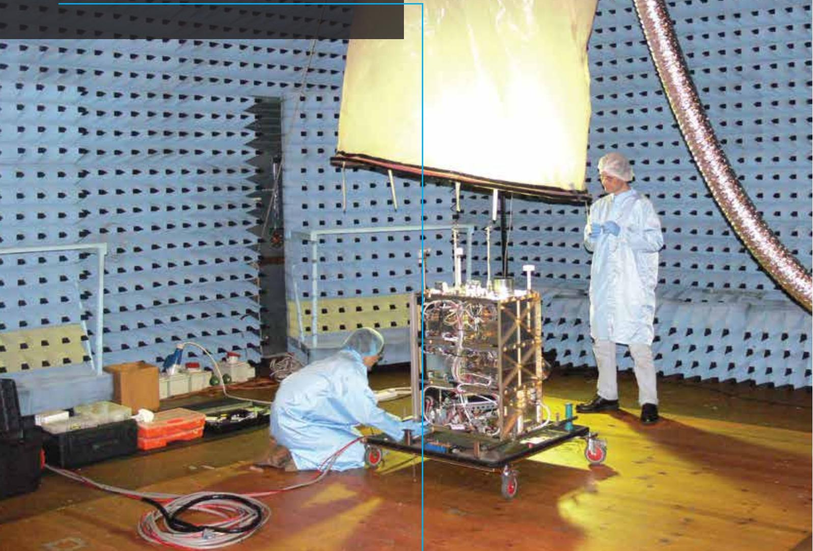
The **EMC Test Facility** at Houwteq provides Electromagnetic Compatibility (EMC) testing services to the commercial, aerospace and defence industries.
